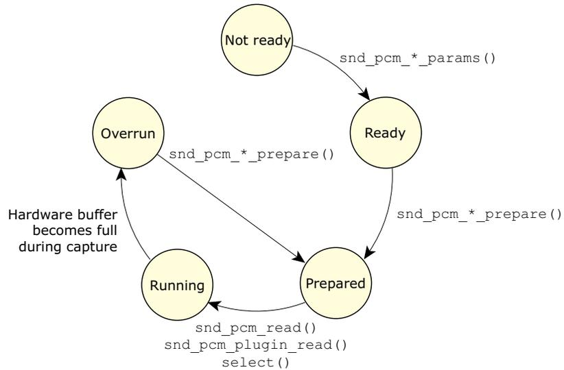
State diagram for PCM devices during capture.
