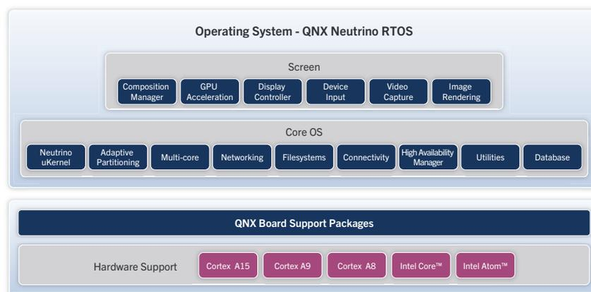
**QNX Neutrino RTOS architecture** – The QNX Neutrino RTOS is a full-featured and robust OS that scales down to meet the constrained resource requirements of realtime embedded systems. Its true microkernel design and its modular architecture enable you to create highly optimized and reliable systems with low total cost of ownership.
