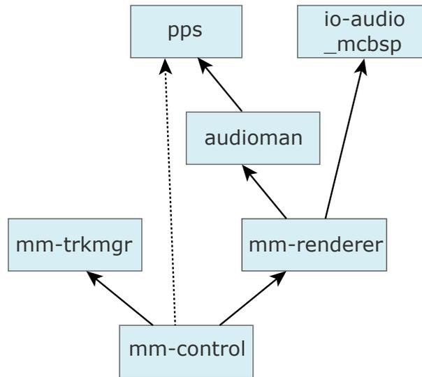
**Figure 1: Workflow of mm-control and related processes**
